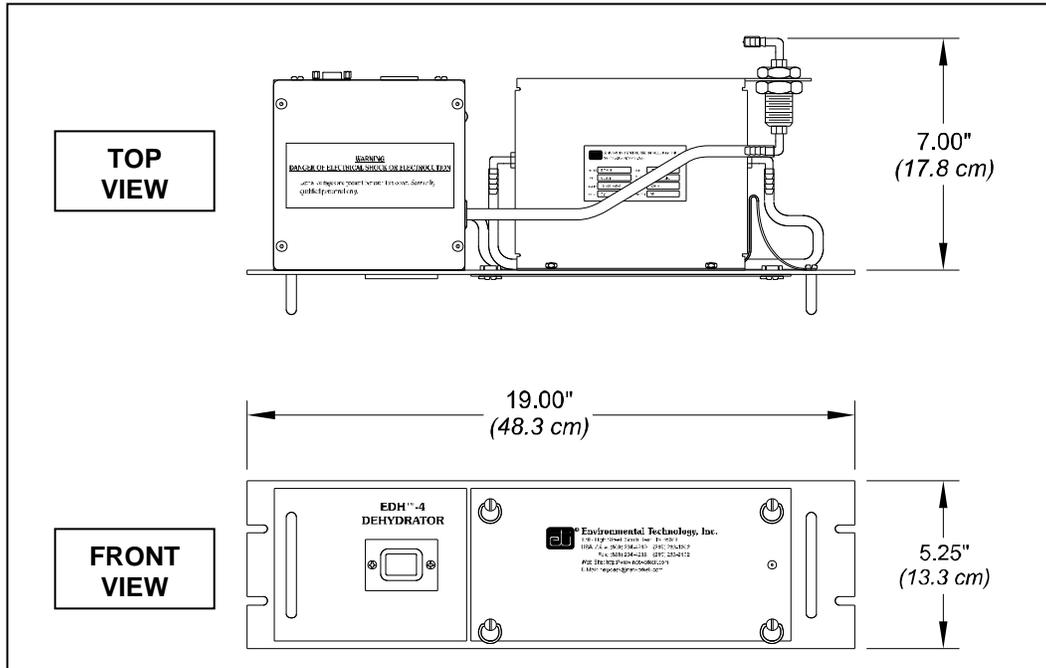
**Figure 2. RACK MOUNTING DIMENSIONS.**
