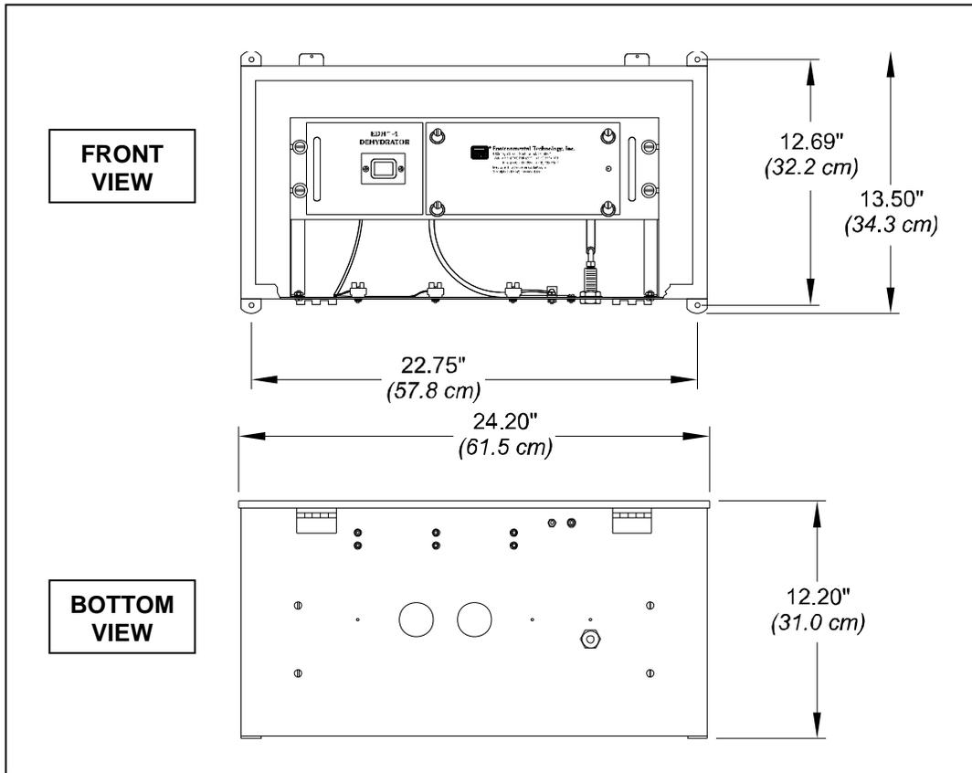
**Figure 4. NEMA BOTTOM MOUNTING DIMENSIONS.**
