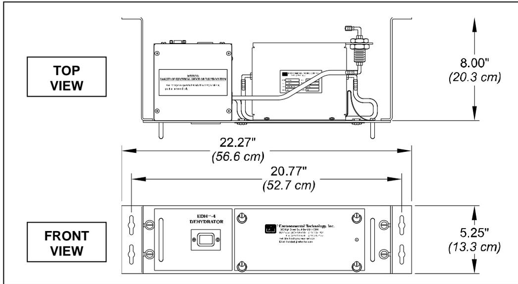
**Figure 3. WALL MOUNTING DIMENSIONS.**
