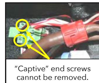
Figure 2. THE POWER CONNECTOR END SCREWS.
