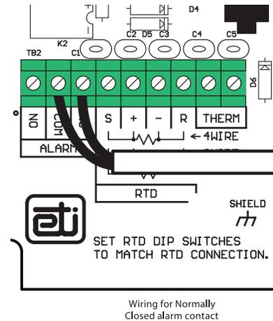
FIGURE 5. External alarm connection
