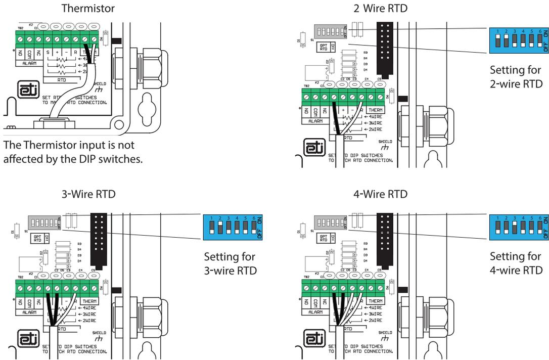
FIGURE 4. Temperature sensor wiring and DIP switch configurations.
